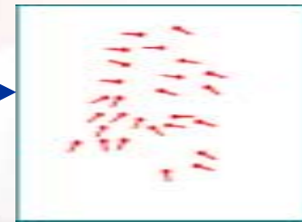
(4) Biometrics traits are extracted and encoded as X,Y coordinates to create a template
